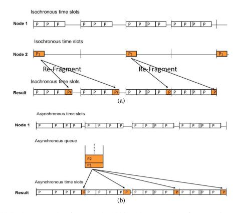
Figure 10: (a) Isochronous packets fragmentation. (b)Asynchronous packets fragmentation.
