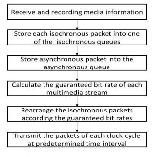
Figure 5: Flowchart of the proposed transmitting network packets
